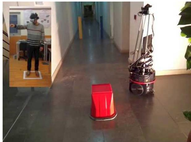
Figure 6. Navigation task, comparison of different teleoperation interaction styles designed to enhance embodiments sensations
